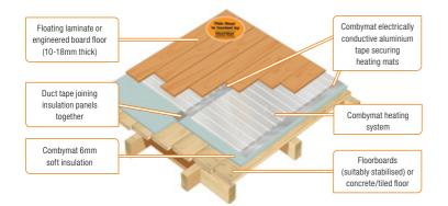
Underfloor heating beneath floating laminate and engineered board floors
